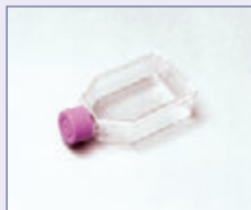
25 cm² culture flask Up to 30 flasks stored in a storage rack Up to 25 observation points in a flask
